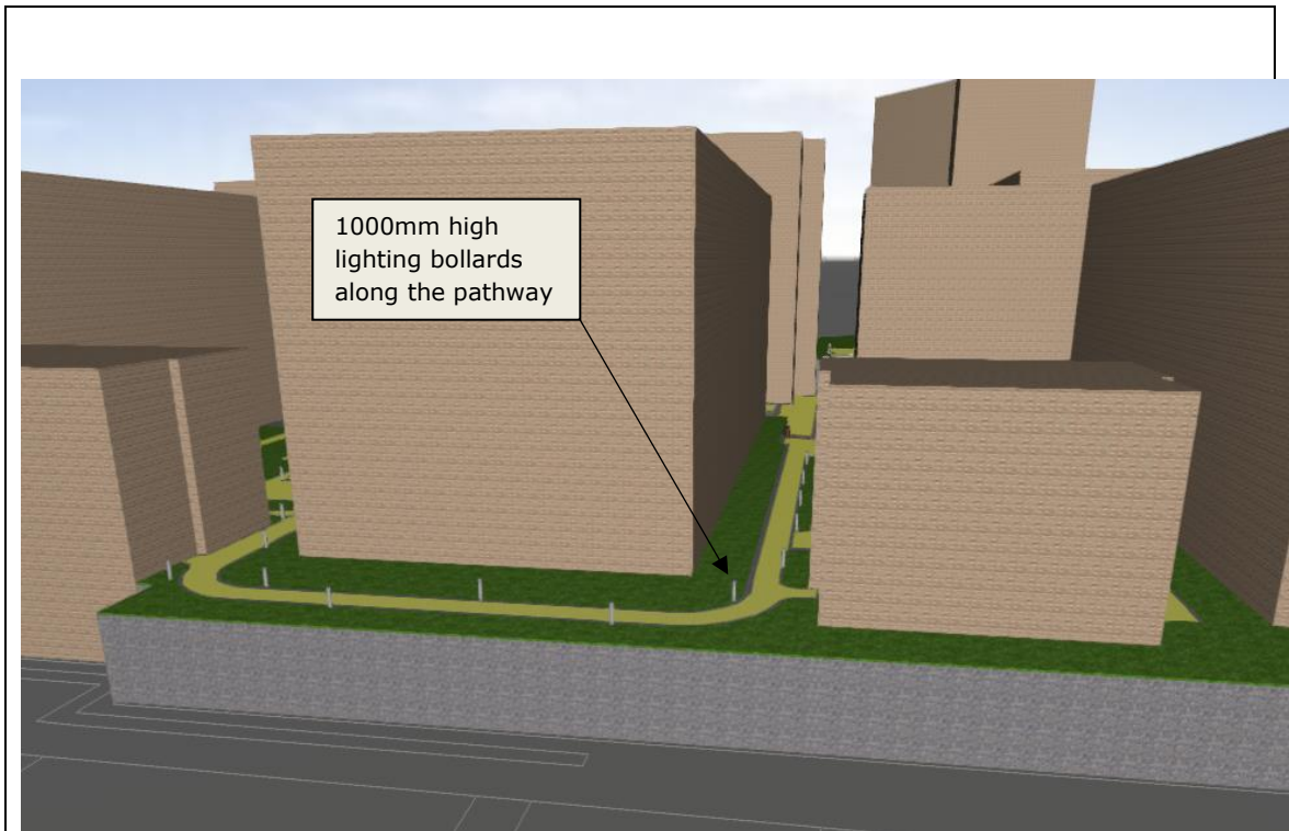
Fig 1 - 3D - Typical Location of Bollard
